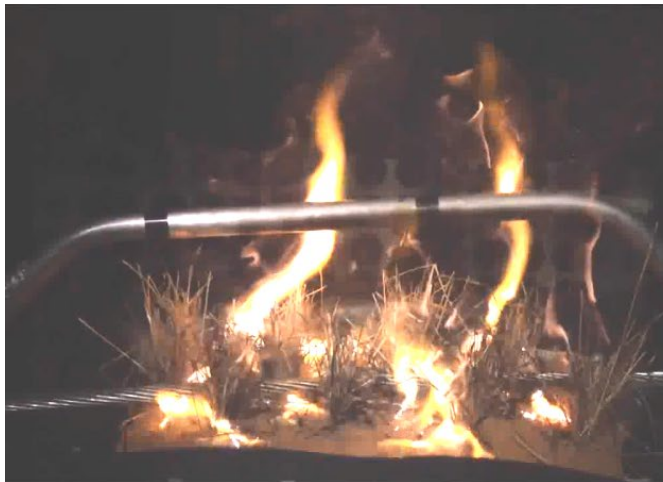
Normal Ground Fault
